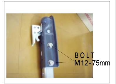
A plate is put in the coupler and the space of the pipe .
